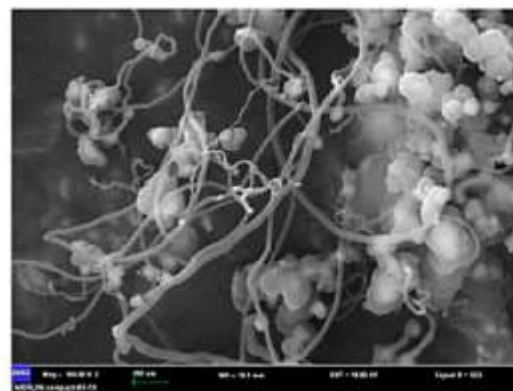
Figure 4. CNT growth on Ni-based catalyst (adapted from [73]).
